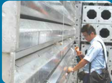
In-house Zinc Coating Thickness Verification
