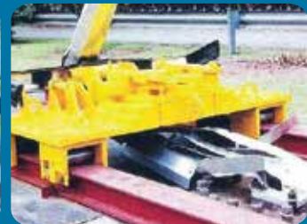
Conclusion of test: The pole does not shear off baseplate, reducing risk of injury
